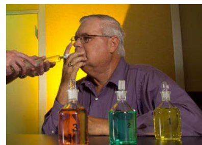
Figure 2. Supplemental Standard odor test. Administration of supplemental standard odor test sample using a mask and glass syringe. Photo ID wstf0807e06127
