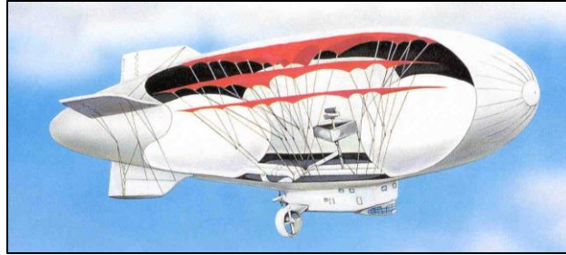
Fig. 1. US Navy YEZ-2A Airship Concept in Showing Internal Structures and Surveillance Radar
