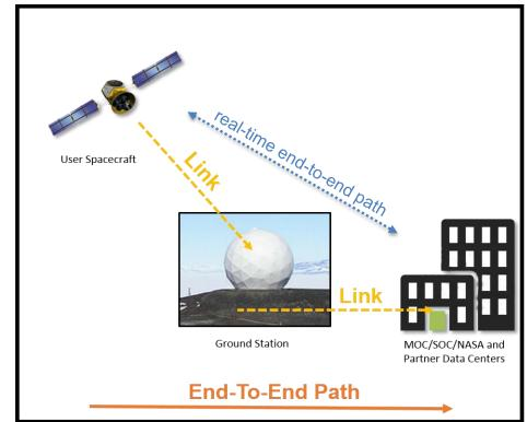
The Space Mobile Network concept leverages the combination of high availability, low latency, low data rate links with delay tolerant users and shared high rate links
