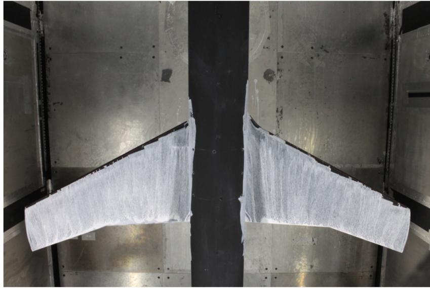
Figure 10. Photograph showing oil flow over both wings (F6 with no horn on port side, F6 with horn on starboard side), \alpha = 5^\circ in the Virginia Tech tunnel (flow is top to bottom).
