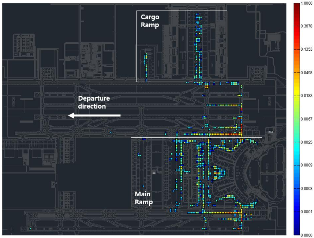
Figure 4. ICN Surface heat map for the stops during the taxi-out phase of north flow departures (April 2015)
