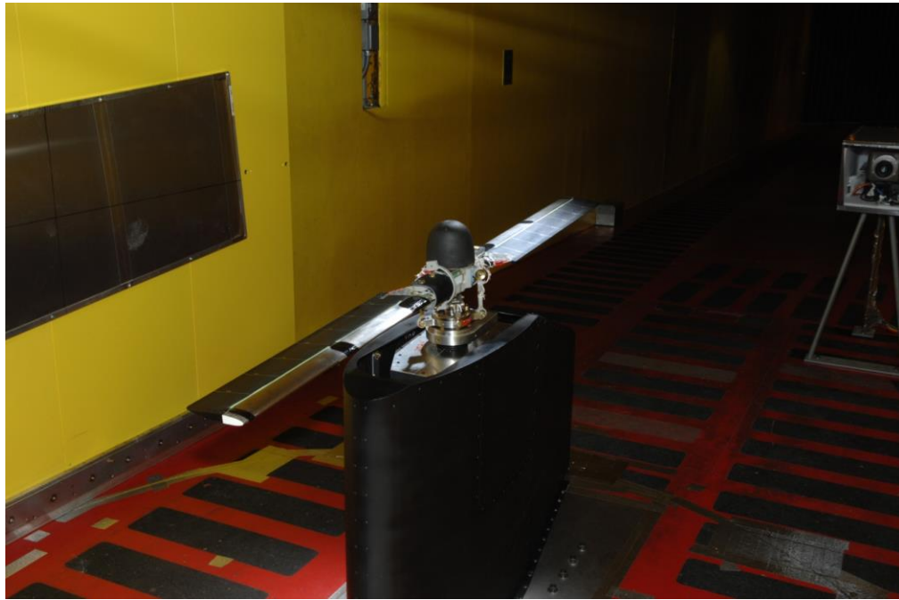
Figure 1. Rotor model in the Icing Research Tunnel.
