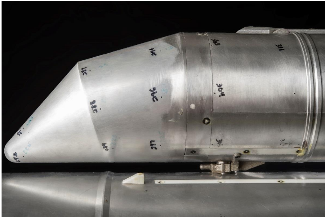
Figure 10. Bent bi-conic nose cone.
