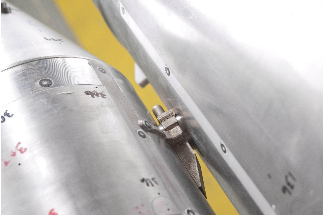
Figure 4. SLS-10005 booster forward attachment protuberance.
