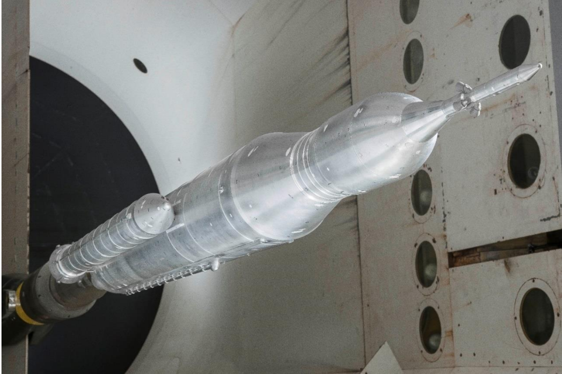
Figure 2. SLS-10005 rigid buffet model installed at TDT.
