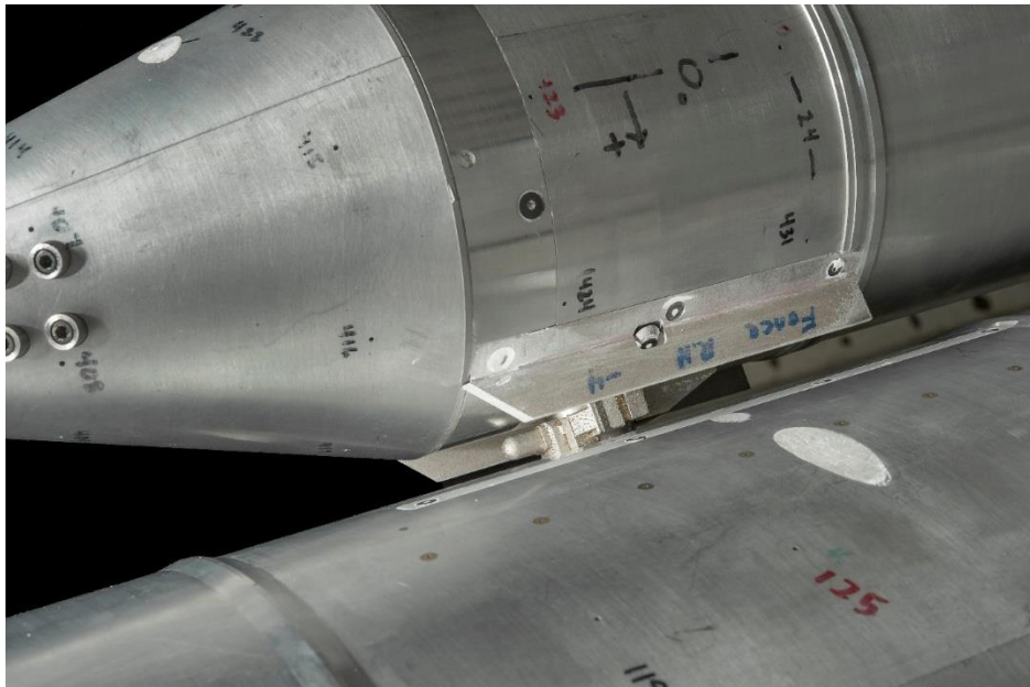
Figure 5. Sharp booster fences.
