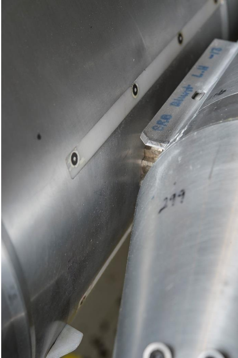
Figure 6. Blunt booster fence (lower fence obscured).
