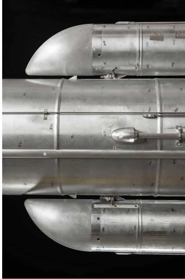
Figure 9. Canted ogive booster nose cones as viewed from bottom of model at 180 deg azimuth.
