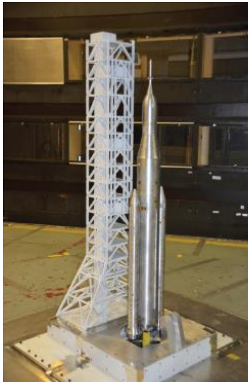
Figure 1. Photograph of model of SLS Block 1 vehicle and launch tower installed in the NASA LaRC 14-by-22-Foot Subsonic Wind Tunnel.
