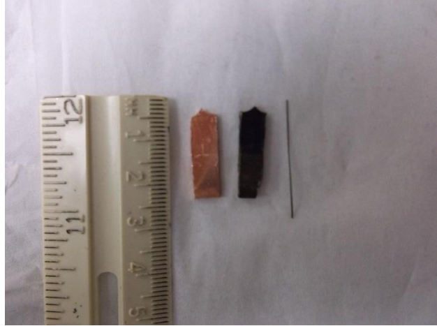
Figure 2. Samples used for thermionic emission. Top side of each shows the pointed end, the bottom side the square ends. The W wire on the right was for reference purposes.
