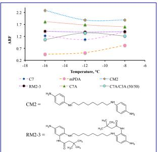
Figure 3. Epoxies containing flexible linkages as pendant and/or in-chain to the polymer backbone.
