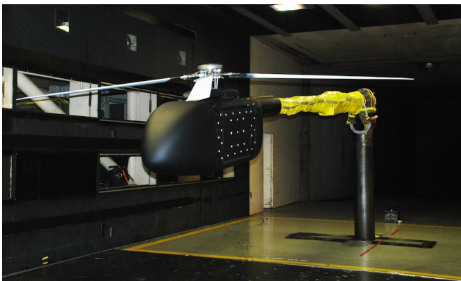
(e) The ROBIN-mod7 model mounted on the GRMS and the long cannon sting.
