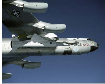
Figure 1. Hyper-X stack being carried to altitude on the NASA B-52B
