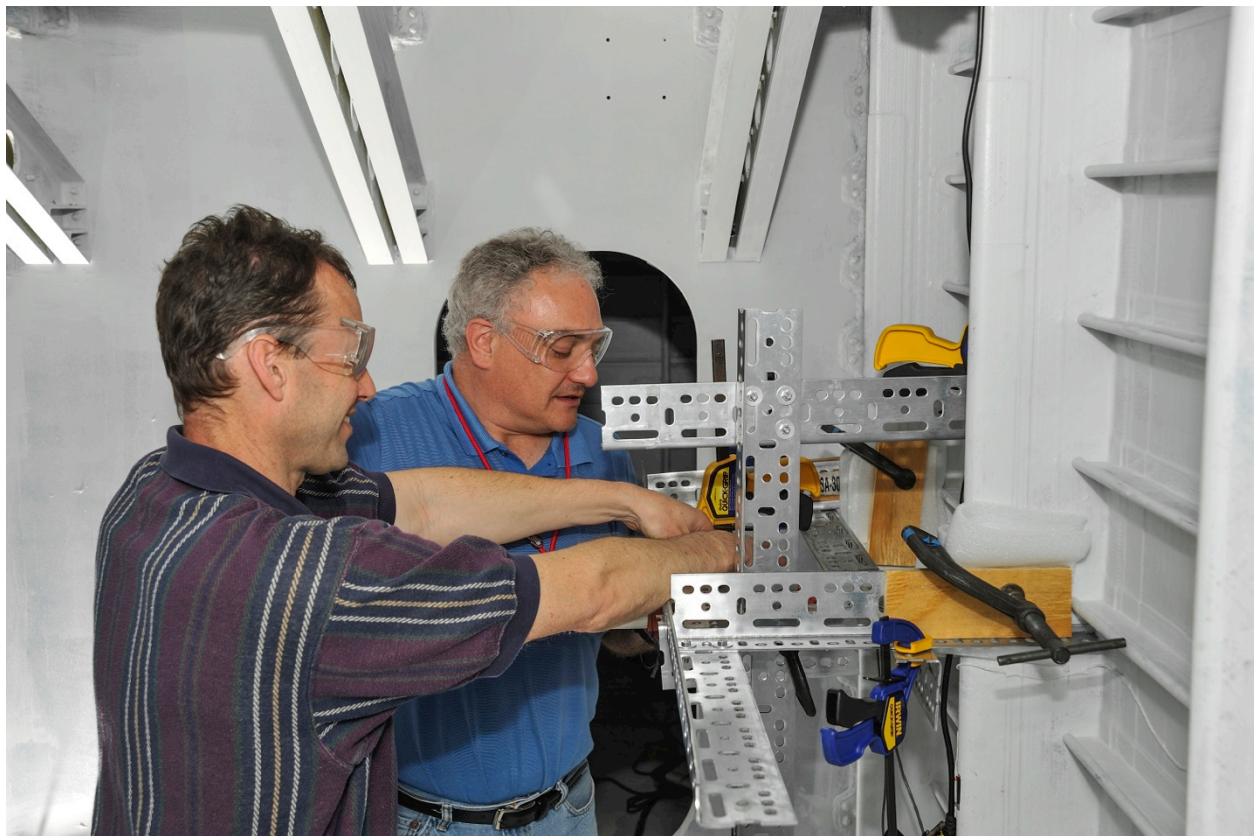
Figure 9. Imparting an interior impact to the MBB skin.
