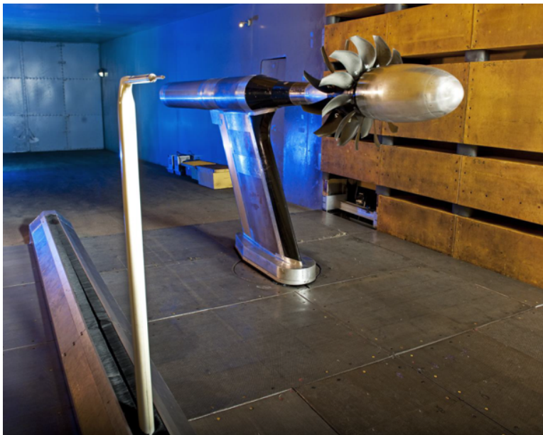
Figure 1: F31A31 test hardware installed in the NASA 9-ft. x 15-ft. wind tunnel.
