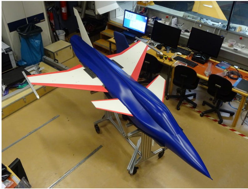
Figure 1: The generic fighter aeroelastic wind-tunnel model to be tested in 2016.
