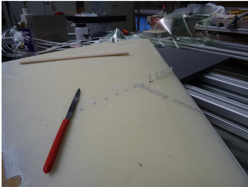
Figure 3: Layout of tubing used for pressure taps in the computer milled molds.
