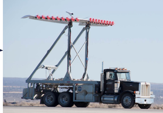
Figure 2: LEAPTech Distributed Electric Propulsion Testbed.
