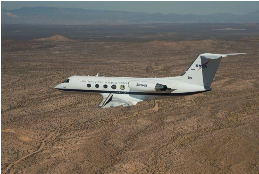
Figure 1. SCRAT airplane in flight with ACTE flaps installed (NASA ED15-076-26).
