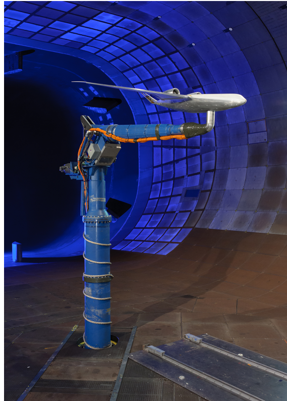
Figure 7. HWB model installed in the NFAC 40- by 80-foot test section with TPS units. (ACD15-0138-002)
