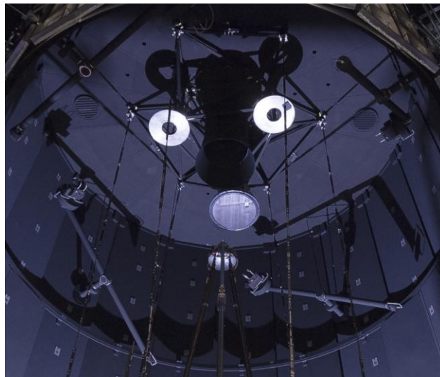
Figure 3 Photogrammetry cameras on windmill booms above the SM and the ACF mirror above the two PMSAs. The COCOA peers through the opening at the center of the ceiling.
