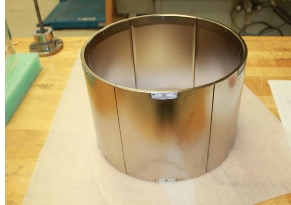
Figure 6. A NiP plated, segmented aluminum pipe with a conical inner figure fabricated for metrology, figuring and superpolishing experiments.
