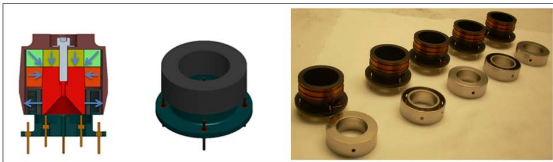
Figure 3. BSM Actuator Cross Section, Bobbin Assy., and Bobbins with Sleeves
