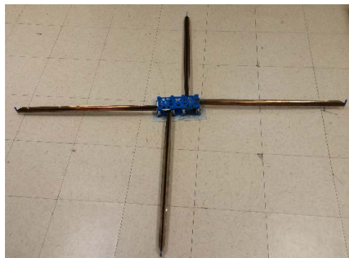
Figure 10. Boom Deployer Prototype with flight-like TRAC booms
