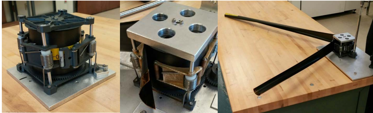
Figure 14. Split Tape Composite Boom Deployer
