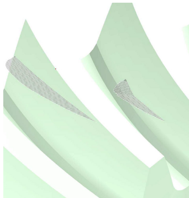
Figure 9.—Instantaneous load intensity drawn on the gear tooth, at 8000 in-lb of gear torque. The load intensity is the load per unit length along the ‘line of contact’. It is obtained by summing up the contact pressures across the width of the contact zone.
