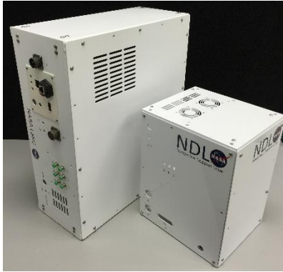
Figure 4. Miniaturized LiDAR chassis developed at NASA Langley in 2012 and 2016
