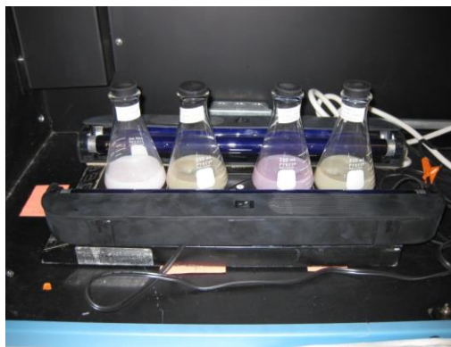
Figure 7: Photodeposition preparation method for quantum dot formation on TiO 2 .
