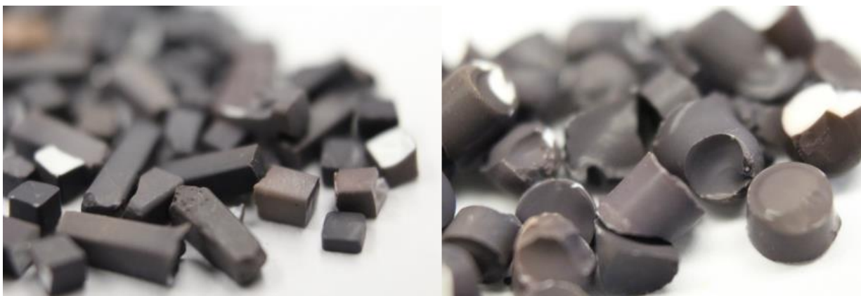
Figure 8: Small (left) and large (right) pellets after direct deposition of silver quantum dots; 3% dopant concentration was based on total weight of pellets rather than TiO 2 in pellet.
