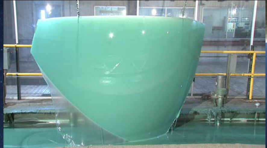
Dome Gore Panel Chemical Milling Los Angeles, CA
