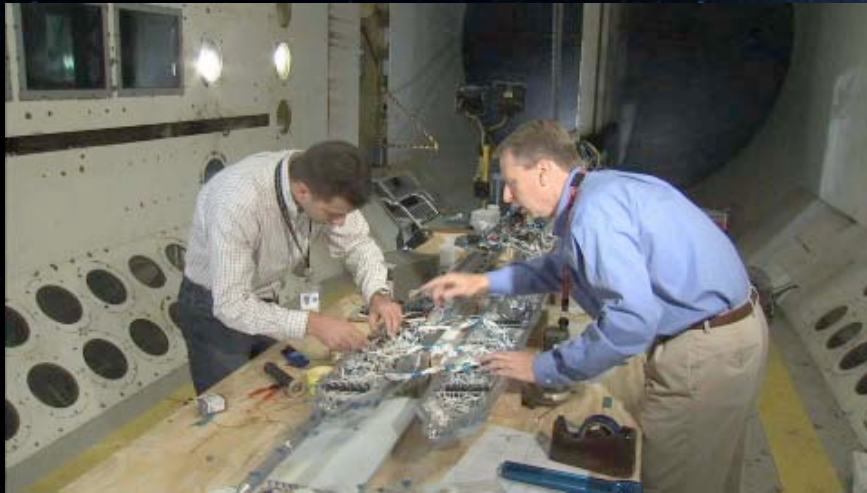
Ares I-X Rigid Buffet Model LaRC, VA
