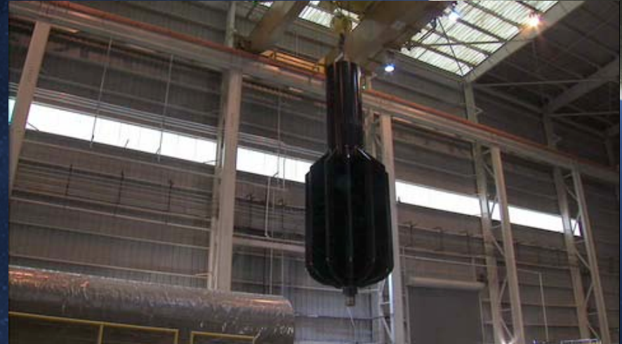
Forward Segment Propellant Core Dry Fit Promontory, UT
