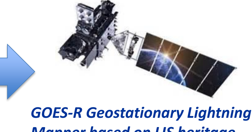
GOES-R Geostationary Lightning Mapper based on LIS heritage
