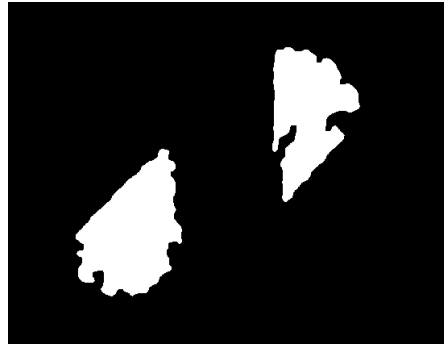
Figure 5. Estimated shape of a delamination from x-ray computed tomography data. The delamination was generated by impacting the composite with a small projectile.
