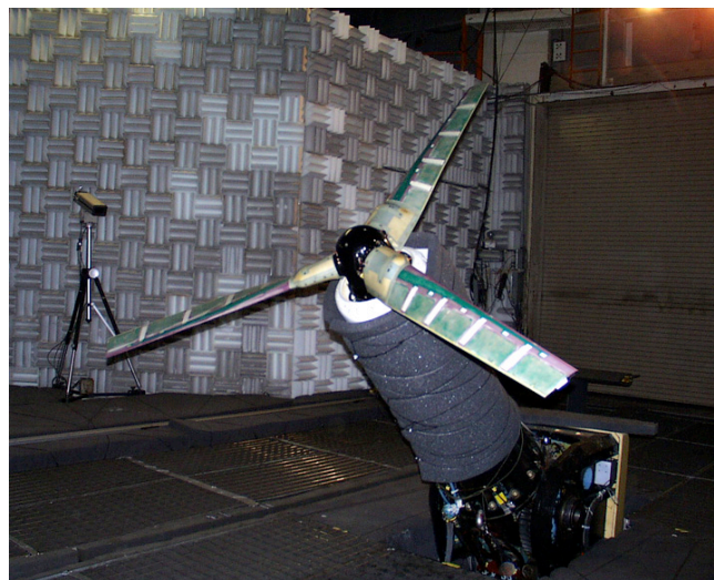
Figure 22. 14 by 22-Foot Subsonic Tunnel open jet with acoustic treatment.
