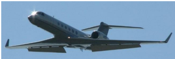
a) 39° deflected flap with main gear retracted, left image 2006 flight test, right image simulated CAD model
