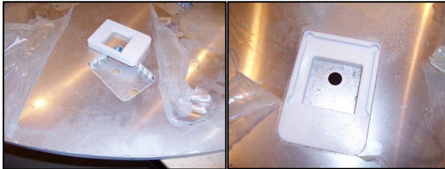
Figure 6. Close-up of central plate construction. Left – Machined aluminum cutout and holder, Right – Assembled unit
