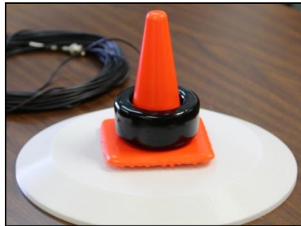
Figure 8. Ground plate assembly. Top – Plate with PCB inserted Bottom – Weighted traffic cone protector
