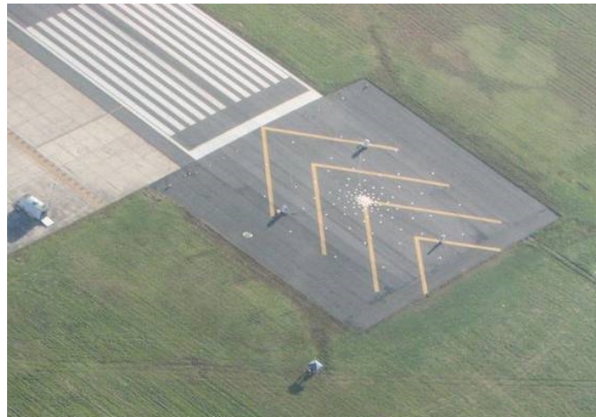
Figure 1. 167-microphone array at NASA WFF in 2006. Dots on overrun area are microphone ground plates. Data acquisition system cabinets are visible around the perimeter of the array.
