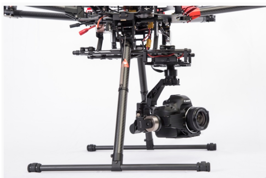
Figure 22. Active gimbal mount for octocopter. (Courtesy DJI)
