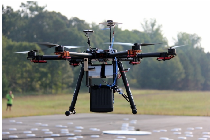
Figure 15. Close up of Langley Hex Flyer in flight with aerial speaker mounted directly underneath.
