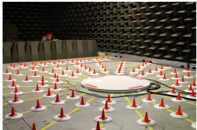
Figure 11. Completed ADL array mock-up.
