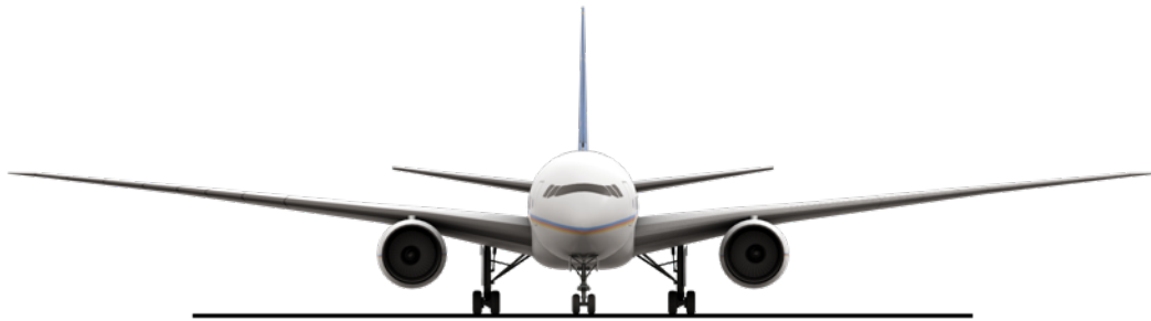
Figure 3. NASA FLOPS optimized 777-200LR-like aircraft concept, front view.
