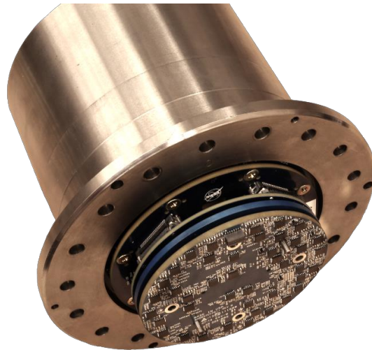
Figure 2. Image of a telemetry system installed on a dummy rotating balance. (Courtesy of Jonathon Ponder at NASA Glenn Research Center)
