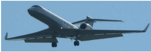
c) 39° deflected flaps with main gear deployed. Left image, 2006 flight test and right image, simulated model.
