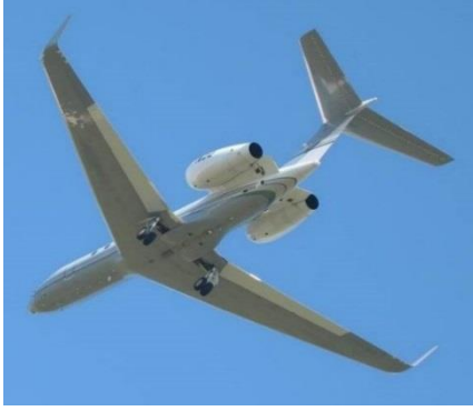
b) 0° flaps (cruise wing) with main gear deployed. Left image, 2006 flight test and right image, simulated model.
