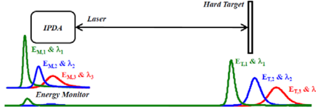
Figure 2. Principle of operation of the 2- \mu\text{m} triple-pulse IPDA lidar for atmospheric CO 2 and H 2 O measurement. The wavelength selection is based on the criteria presented in figure 1.
