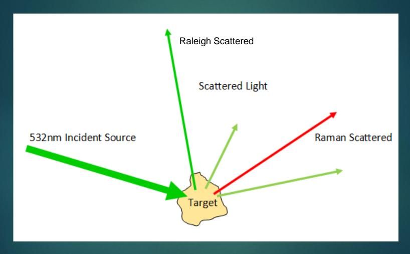
Example of photon behavior when hitting polarizable material
