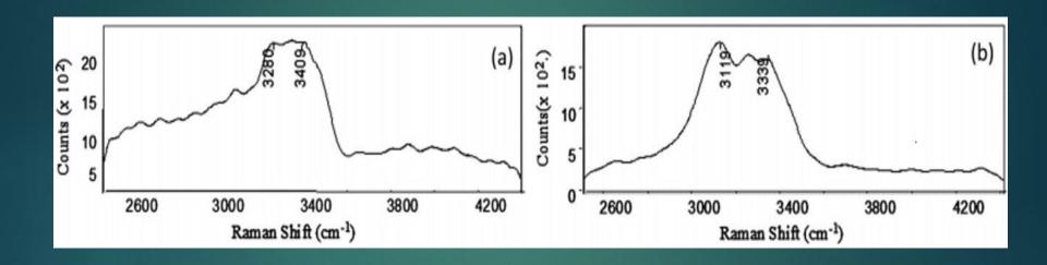
Example Raman spectra of (a) water, and (b) ice [2]
