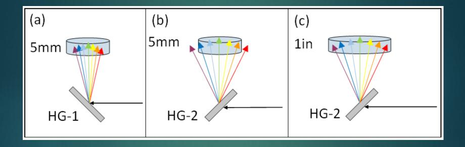
(a) Reflective grating with 5mm collection lens capturing full spectrum,
