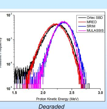
50.8 μm aluminum & 3.175 μm Mylar Degraded proton beam energies
