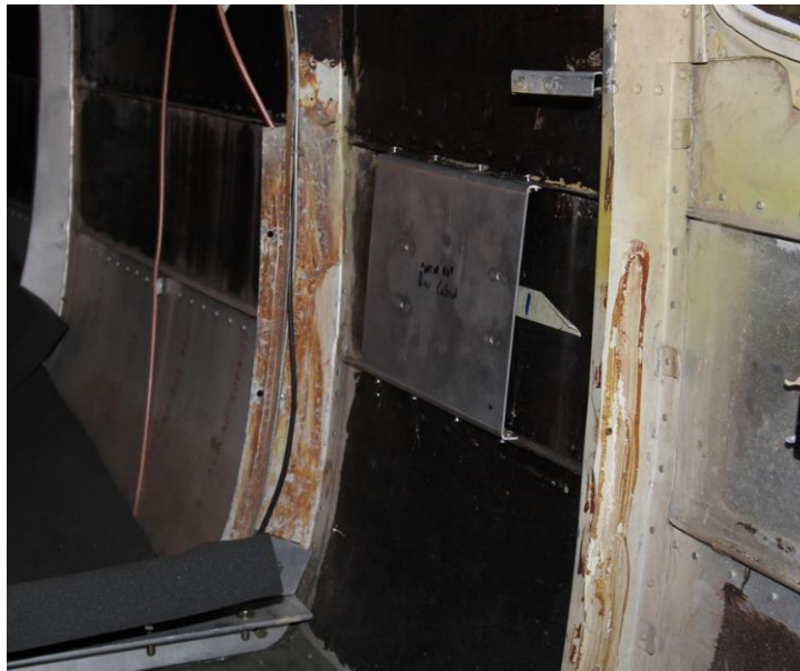
Figure 4 - Example sidewall aircraft attachment plate
