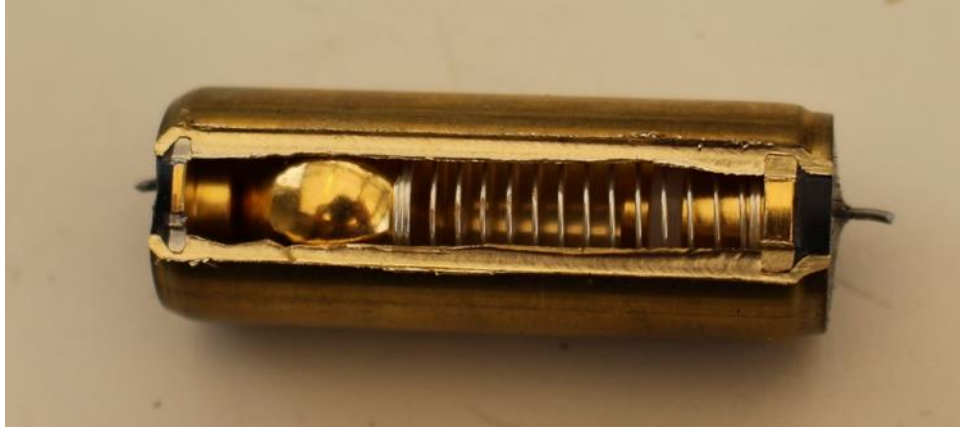
Figure 24 – G-switch assembly for ELT beacon 4 on Test 2
