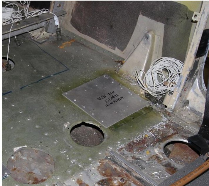
Figure 3 – Example floor mounted aircraft attachment doubler plate
