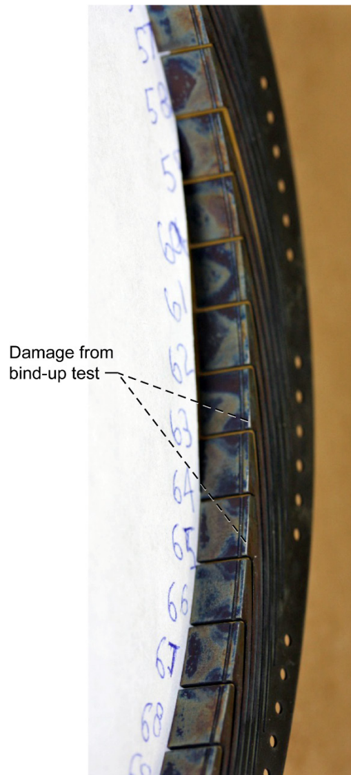
Figure 24. Build 1 non-contacting finger seal aft finger lift pads inner diameter surface after static performance testing at 922 K.
