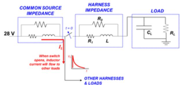
Figure 8. Typical Turn-Off Transient
