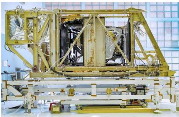
Figure 3. ISIM Installed in Mounting Frame
