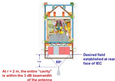
Figure 9. Field Levels at Rear Face of IEC
