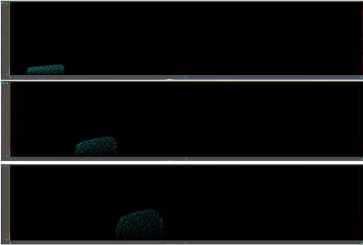
Figure 3.3.2-1 – PIC simulation of a traveling \alpha -particle bunch in cylindrical geometry.
