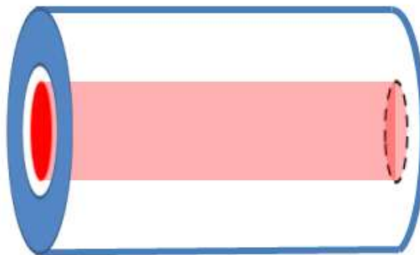
Figure 3.4.3-3 –Capacitive coupling of the bunch passing through a long TWDEC electrode: coaxial cable approximation
