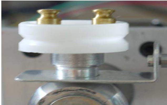
Figure 5.12 10g total force on top of the substrate aluminium substrate and aluminium sample.
