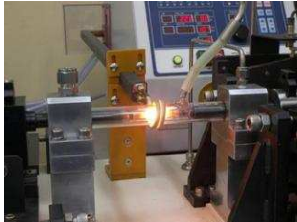
(b) heating by induction heater
