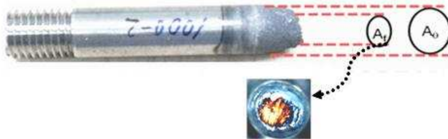
Fig.3.9 Geometry of sample after fracture.
