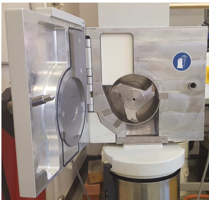
Figure S2. Image of the cutter mill used for cocrystal particle size reduction.
