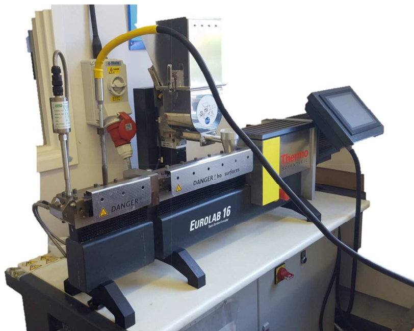
Figure S1. Image of a twin – screw Eurolab 16 extruder use for continuous cocrystallization processing.
