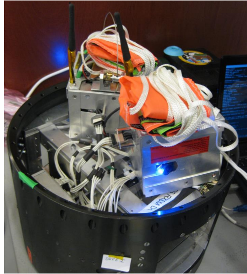
Figure 12: CubeSat Modules being tested while sitting on experiment housing
