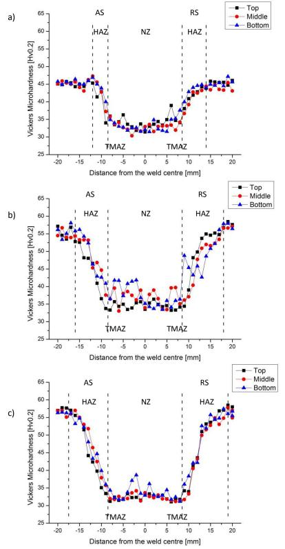
Fig. 5. Microhardness profiles for (a) '0' joint, (b) '4' joint, (c) '8' joint
