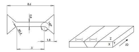
Fig. 1. Schematic illustration of tensile specimens together with their locations in butt welded plate (JD – joining direction along length of the plate)
