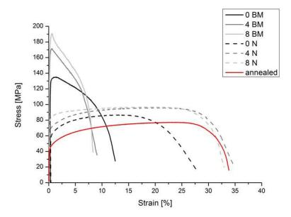
Fig. 6. Stress-strain curves for tensile specimens cut from base material (BM - solid lines) and nugget (N- dashed lines) for 0, 4 and 8 IECAP passes; red line – annealed material
