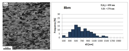
Fig. 2. Representative microstructures of base materials: (a) initial state, (b) after 4 and (c) after 8 passes of IECAP (X plane perpendicular to welding line) together with histograms of grain sizes  $(d_2)$
