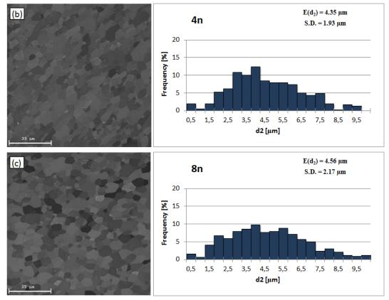
Fig. 4. Representative microstructures of nuggets in: (a) '0', (b) '4' and (c) '8' samples together with grain size  $(d_2)$  histograms
