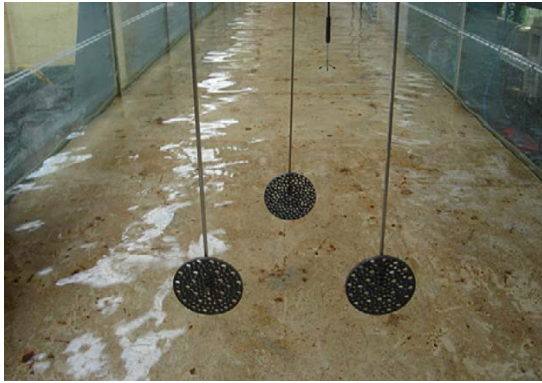
Figure 9 Actuator disks used to simulate turbine arrays in flume tank tests (Myers and Bahaj, 2011)
