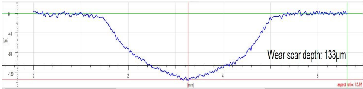
Figure 5. Surface profile scan of the wear scar of the medium carbon steel UNS G10400 after solid/liquid impingement.
