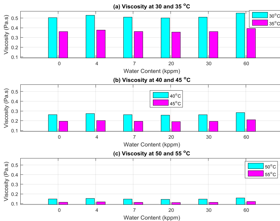
Figure 8.2 Viscosity with different water contents at different temperature values
