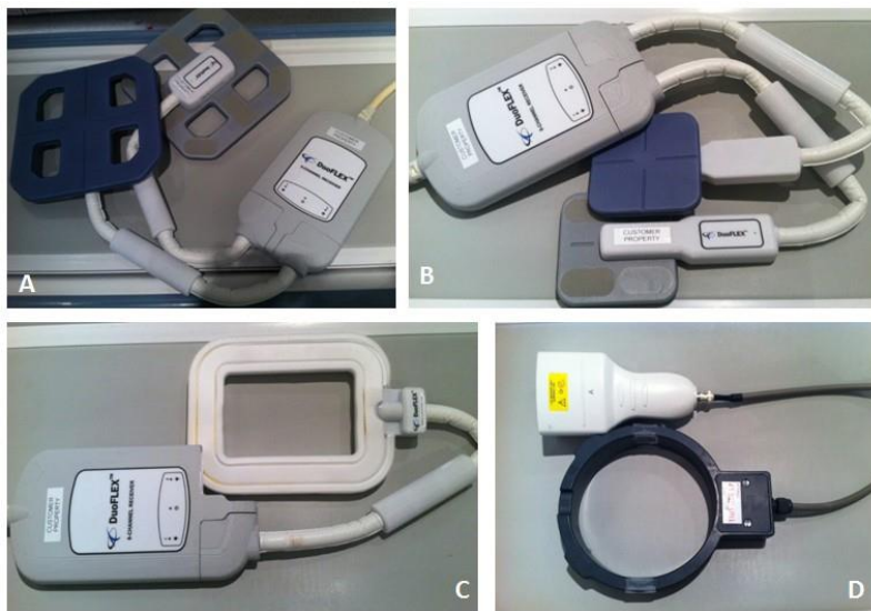
Figure 6.5 DUOFLEX interventional 8-channel phased array coil 24 \times 24 cm (A) and 10 \times 10 cm (B); DUOFLEX interventional single channel coil (C); and InSightec 5GP breast coil (D).
