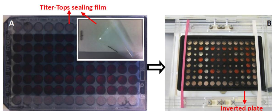
Figure 5.8 96-well plate fully filled with medium and sealed with Titer-Tops ® sealing without air-bubble formation (A); Inverted plate with \mu clear bottom fixed in sonicator by plate holder and further fixed by rubber bands in both sides (B).
